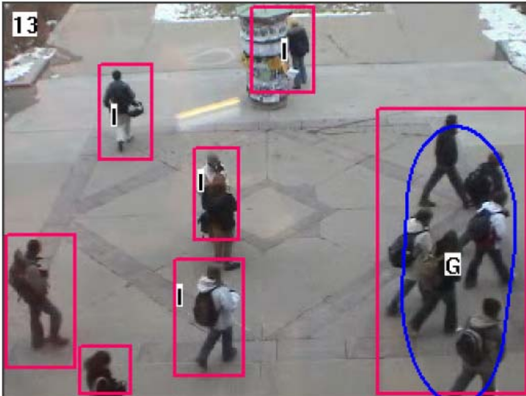
Fig. 14. A sparsely populated group with a small tilt angle. Note that the system slightly overestimates the count owing to big gaps in the group.
