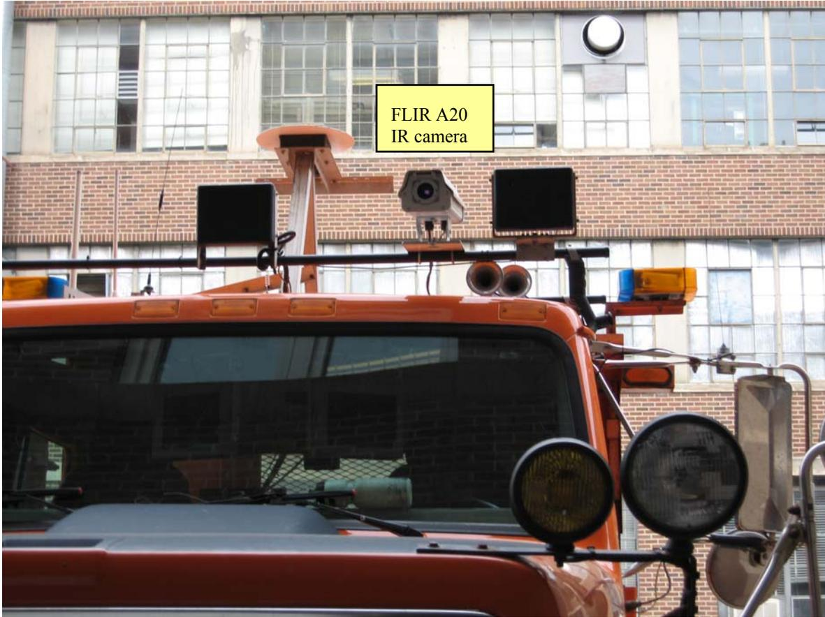
**Figure 4. FLIR A20 IR camera on the Safeplov**
